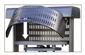
Once the compression is complete, the lower disc descends to its initial rest position.
